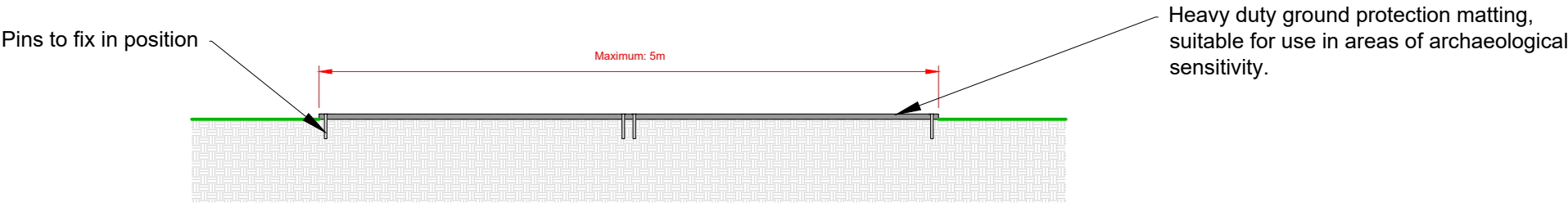
ILLUSTRATIVE SECTION THROUGH TEMPORARY ACCESS TRACK
